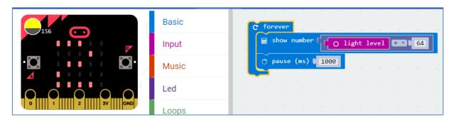
Don't bother saving, downloading and transferring (aka `flashing') the current program to your micro:bit. We can now merge this idea with our 4-state program, replacing the `button' test with a `light level' test. We will now introduce the idea of a `variable'. In the
